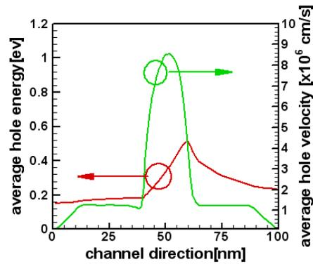
Figure 2: Hole energy and velocity in the direction of transport from source to drain, both averaged over the entire silicon body of the p-FET with  $V_g = -1.55$  V and  $V_d = -1.0$  V.
