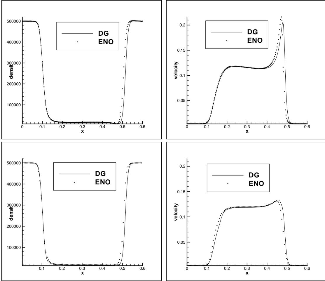
Figure 1: Comparison of the discontinuous Galerkin method (solid lines) with the finite difference ENO method (symbols) for a one dimensional silicon  $n^+-n-n^+$  diode of length  $0.6\mu m$ . Top: hydrodynamic (HD) model; bottom: energy transport (ET) model. Left: electron density  $n$  ( $10^{12}cm^{-3}$ ), right: velocity  $v$  ( $\mu m/ps$ ).
