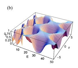
**Fig. 2.** (a) Geometry of an asymmetric ring with an attractive potential dot. The lengths of upper and lower arms are  $L_u$  and  $L_d$  correspondingly, and  $L_s$  is distance of the dot from left junction. (b) 3D plot of electron transmission through the asymmetric ring, showing variation with electron energy and threaded magnetic flux.
