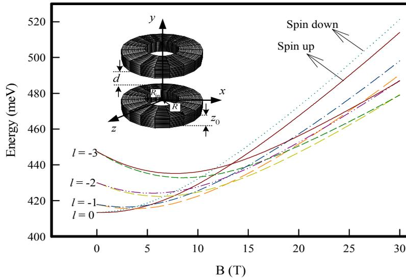
Figure 1: Electron energy spectra for vertically 2-coupled InAs/GaAs quantum rings with  $d = 0.8$  nm.
