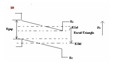
Figure 1: (A) Bandbending due to spontaneous polarization in the presence of electrolytic screening; (B) Bandbending due to spontaneous polarization with no electrolytic screening.
