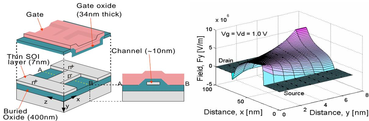
**Figure 2:** **Left:** The device structure of the 10nm SOI MOSFET. **Right:** The  $y$ -component of the field due to the boundary conditions,  $F_y$ , within in the device for  $V_g = V_d = 1.0\text{ V}$ .
