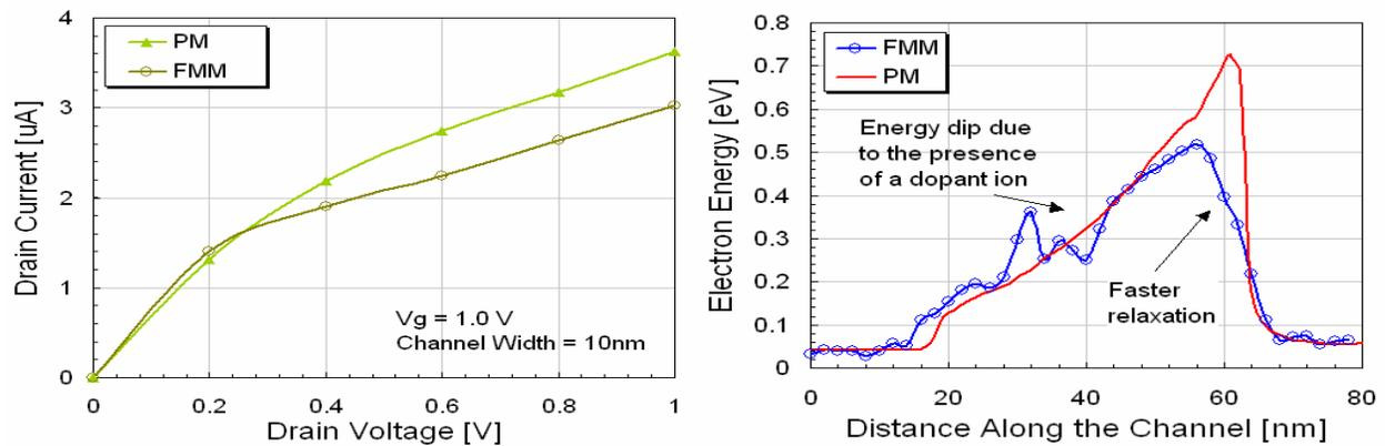
**Figure 3:** **Left:** The  $I_d - V_d$  curve for a gate voltage of  $V_g = 1.0\text{ V}$  as obtained by the PM and FMM methods. **Right:** The electron energy along the channel for the PM and FMM approaches.
