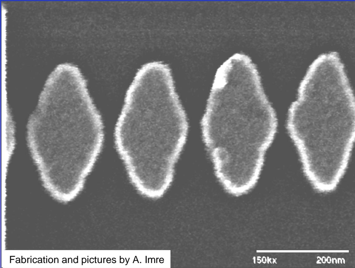
Investigations of permalloy nanomagnets (thermally evaporated and patterned by electron beam lithography) confirm the simulation results
