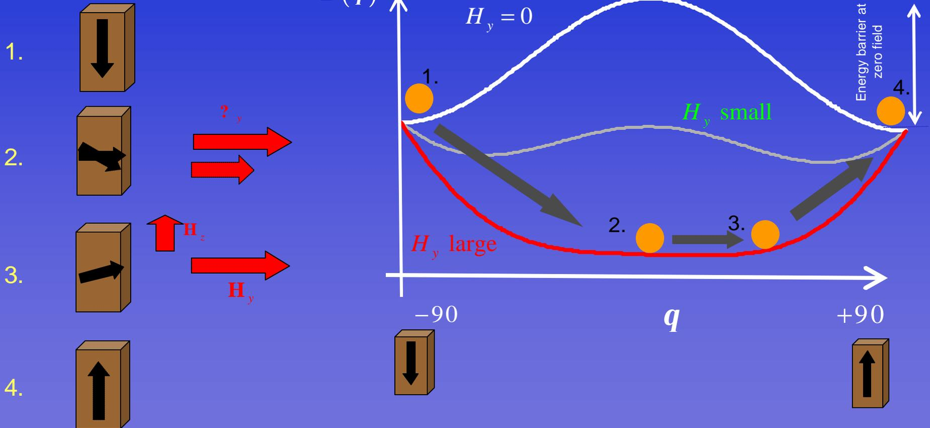
By adiabatic clocking, the system can be switched with almost no dissipation, but at the expense of slower operation.
