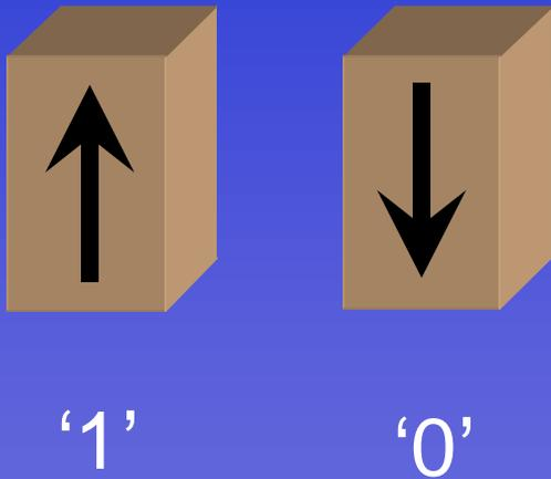
Due to shape anisotropy there is a typically few hundred room-temperature  $kT$  energy barrier between the two stationary states.
