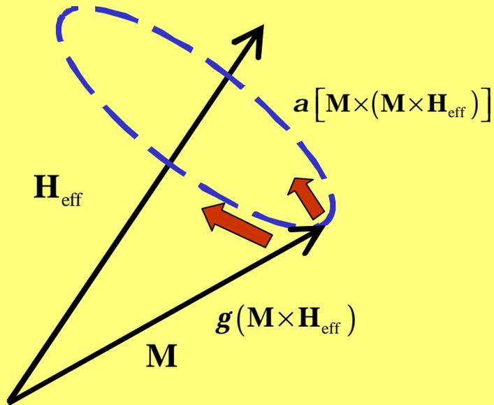
Magnetic moments (spins) of the ferromagnetic material perform a damped precession motion around the effective field.
