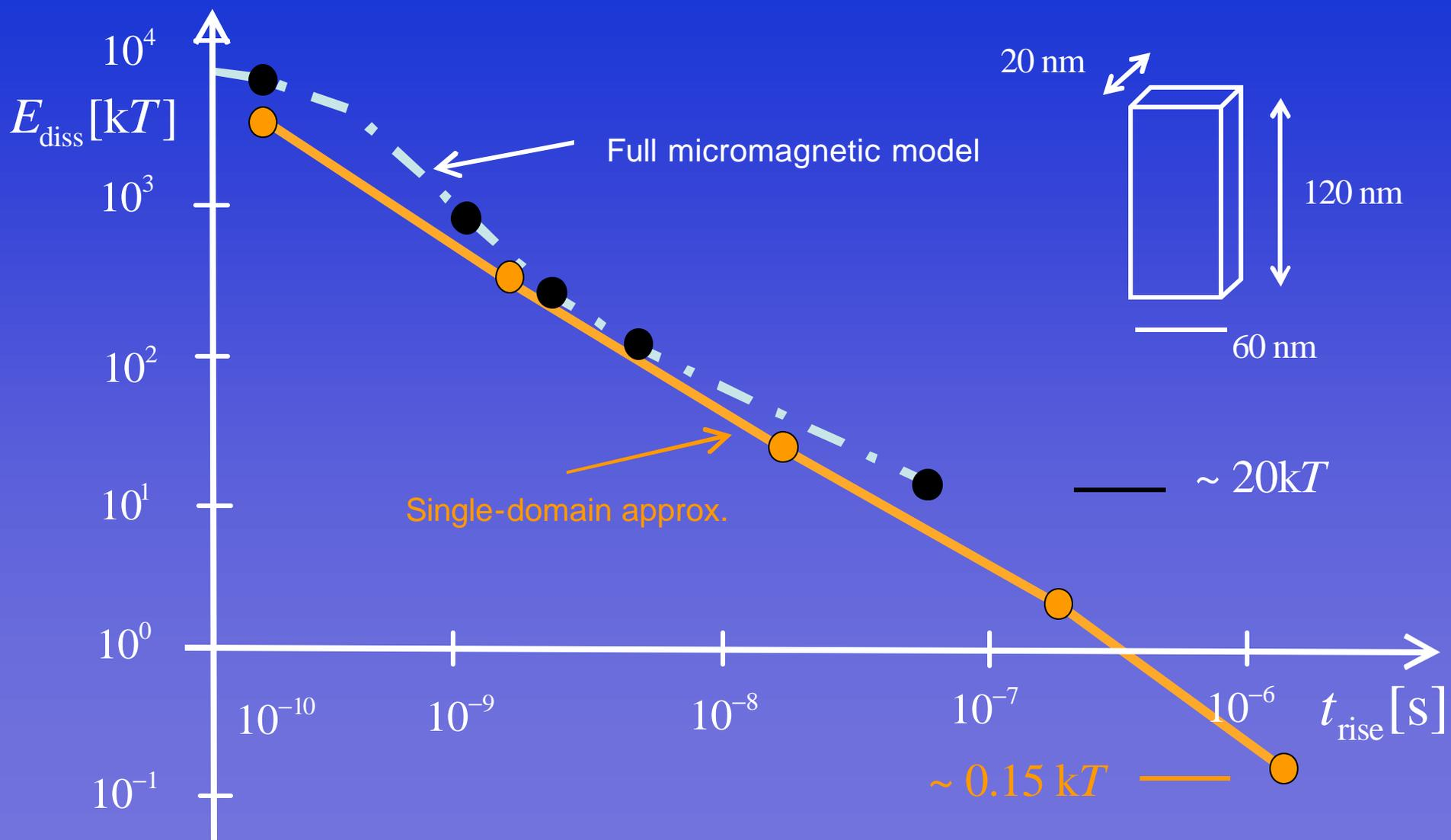
Adiabatically switched nanomagnets can dissipate at least two orders of magnitude less energy than the height of the potential barrier separating their steady-states
