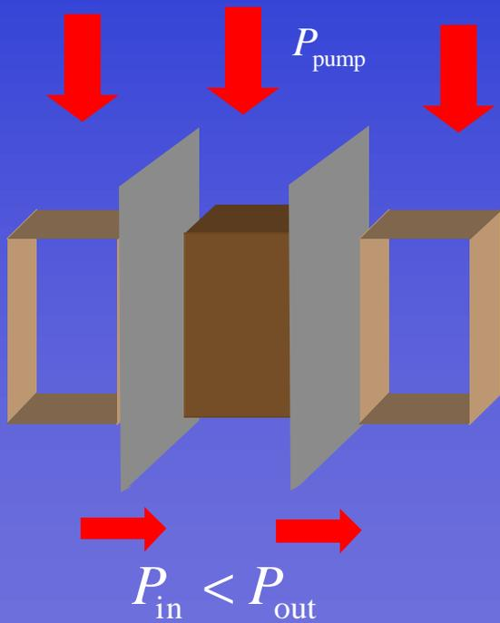
Energy of the magnetic signal increases as the soliton propagates along the wire
