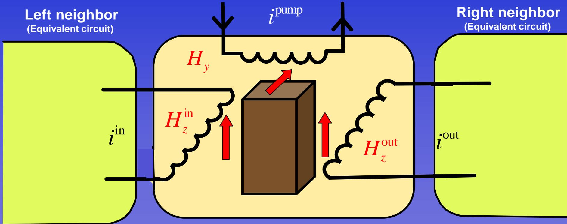
The origin of power gain in field-coupled nanomagnets can be understood on the same basis as the operation of magnetic parametric amplifiers
