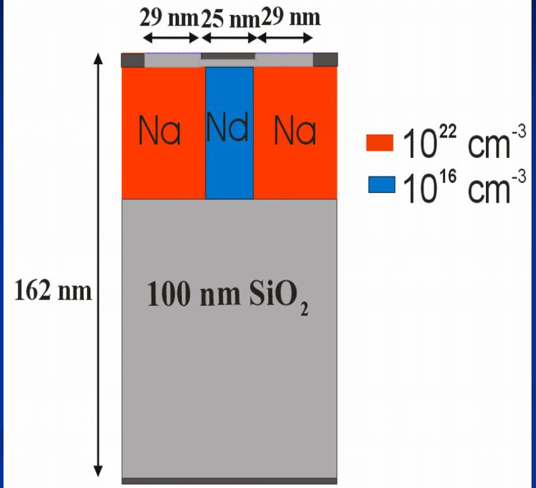
➤  $H_{\text{si}} = 50 \text{ nm}$  ,  $W_{\text{si}} = 25 \text{ nm}$  ,  $L_g = 25 \text{ nm}$ , doping
