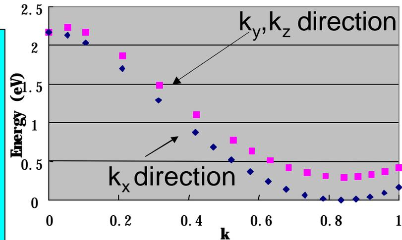
Band structure of conduction band near X point with 50% expansion of  $k_y, k_z$  direction.
