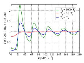
Fig. 2: Transmittance at resonant frequency (200 THz) of ideal two level atom from [1] for different electrical field amplitudes when dephasing time  $(T_2)$  is larger, equal and smaller than signal width  $T_{\rm P}$ . Oscillations at  $E_0^{2\pi} = 21$  MV cm<sup>-1</sup> can be clearly observed.
