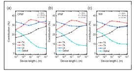
Fig. 6. Spectral contributions of each phonon mode to the total heat flux as a function of length for (a) CPNF, (b) IPNF, and (c) NW at 300 K.
