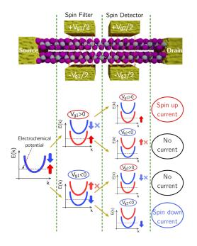
Fig. 1. (Top) Schematic of the device architecture. (Bottom) Pictorial sketch of the spin-polarized bottom of the conduction band structure for the filtering and detecting mechanism for different values of  $V_{g1}$  and  $V_{g2}$ .
