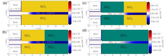
**Figure 1**. Color plots of free charge density for the four dielectric combinations. The TMD is *n*-doped to  $1.73 \times 10^{13}$  cm<sup>-2</sup>. Configurations with low- $\kappa$  environment closer to metal edge have smaller depletion widths.
