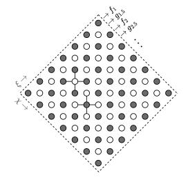
Fig. 1. Illustration of the staggered grid composed of the two subgrids (f-black and g-white) in the center-of-mass coordinates  $\chi$  and  $\xi$ . The circles stand in for the elements of the density matrix. The coupling between the two grids is indicated for two grid points. When not at the boundary each element couples to four neighboring elements.
