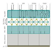
Fig. 1. Sketch of the stacked structure considered. The arrows represent the behavior of light beams according to each model.
