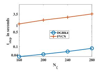
Fig. 5: Comparison of the computation time between the DGRK4 algorithm and the FV-Crank Nicolson (FVCN) scheme [5].  $N_{\xi}$  indicates the number of  $\xi$ -elements.
