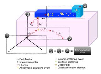
Fig. 1. Sketch of the physical processes within the DM phonon based detector. The related and individual processes—(1) DM -target interaction, (2) phonon downconversion, (3) interface scattering, and (4) pair breaking diffusion and detection—that affect the detected signal are indicated with black-dashed boxes.
