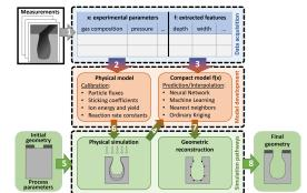
For model generation, experimental data (1) is used Fig. 4. to calibrate physical models (2), while a compact model is trained using experiments (3) and physical simulations (4). A simulation from initial conditions (5) can use a physical model (6) or a compact model (7) to obtain the final geometry (8).
