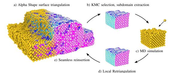
Fig. 1. Circular coupling method of the atomistic vapor deposition model: a) Global triangulation and Alpha Shape construction of the active surface b) KMC sampling of adsorption events at the active surface c) MD simulation around the adsorption site d) Local retriangulation of the subdomain e) Seamless reinsertion due to a shared domain boundary and the alpha criterion
