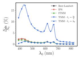
Fig. 5. Comparison of the four models in the visible range. While TMM overlaps with the rest of models for  $t_{\rm subs} = \lambda_0$ , it approaches a resonance when  $t_{\rm s} \approx \lambda_0/2$ , for which  $N_{abs}$  increases in a factor of about 10.
