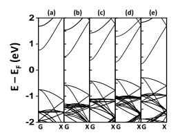
Fig. 3. Band structures of (a) GaAs, (b)  $In_{0.25}Ga_{0.75}As$ , (c)  $In_{0.5}Ga_{0.5}As$ , (d)  $In_{0.75}Ga_{0.25}As$  and (e) InAs.
