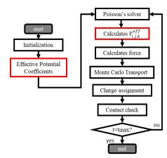
Fig. 1. Flowchart of the quantum corrected MC simulator.
