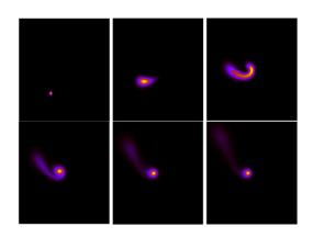
Figure. Time evolution of the probability density of finding a skyrmion which is approaching a pinning site at 150 K.
