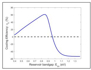
Fig. 6. The cooling efficiency  $\eta_{cooling}$  is shown with ideal II as a function of the reservoir bandgap  $E_{cv}$ . The black dashed line stands for  $\eta_c = 0$  %.
