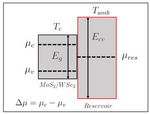
Fig. 3. Band diagram of our device where the MoS<sub>2</sub>/WSe<sub>2</sub> heterojunction (bandgap  $E_g = 0.4 \text{ eV}$ ) is in contact with a reservoir (bandgap  $E_{cv} \ge E_g$ ).  $\mu_c$  ( $\mu_v$ ) is the Fermi level of electrons (holes) in the conduction (valence) band.  $\mu_{res}$  is the Fermi level in the reservoir.  $T_c$  is the carrier temperature in the heterojunction.  $T_{amb} = 300 \text{ K}$  is the ambient temperature.
