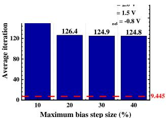
Fig.4. Distribution of the number of iterations for 1,000 devices, when the proposed method is applied at  $V_G = 2.0$  V,  $V_D = 1.5$  V, and  $V_{BB} = -0.8$  V.
