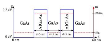
Fig. 2: Schematic representation of a resonant tunneling diode showing the band edge potential and the spatially varying effective mass  $m_0$ .
