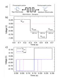
Fig. 4: a) Pre- and post-synaptic pulses were applied to the top and bottom memristor electrodes, respectively b) voltage waveform (cycle) applied to measure the set and reset currents (20 times) for a given Vset. (c) Amplitude and duration of Vset has been changed by delaying the post-synaptic pulse. Solid lines: pre- and post-synaptic pulses, without overlapping. Dashed lines: examples of delayed post-synaptic pulses.
