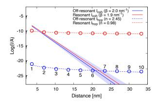
Fig. 3. Distance dependencies of coherent  $(I_{coh})$  and incoherent  $(I_{hop})$  current in multi-STC junctions. [6]
