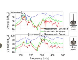
Fig. 4. Comparison between Simulated and Measured Frequency Characteristics with Adjusted Indenter Length
