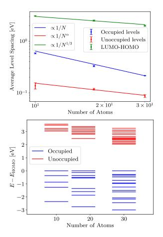
Fig. 2. Scaling of various charged excitations of metallic clusters in evGW. Top: average level spacings and gaps in an ensemble of metallic clusters as a function of the number of atoms. Lines are guides to the eye; they reveal that the HOMO-LUMO gaps scale with a slower power law, leading to HOMO-LUMO widening. Right, the energy levels of sample clusters is shown, with HOMO aligned to 0.
