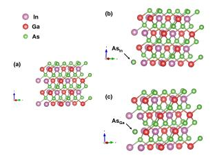
Fig. 4. Relaxed atomic structures of (a) defect-free, (b) w/  $As_{In}$  and (c) w/  $As_{Ga}$  in  $In_{0.5}Ga_{0.5}As.$
