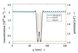
Fig. 3. The electron density from the use of TB-QLTE for one of the both grids is shown as a function of the coordinate  $\chi$ . For the equilibrium case, the results are compared to those obtained from the NEGF method. The results agree very well. For the k-discretization  $N_k = 200$  values were considered.
