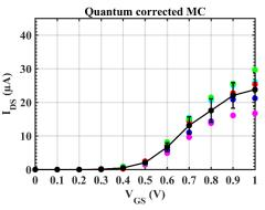
Fig. 5. Transfer characteristics obtained with the QC MC simulator for five devices with different random dopant distribution in the source, drain and channel. The average channel doping is  $10^{15}$  cm<sup>-3</sup>. V<sub>B</sub> = V<sub>S</sub> = 0 V and V<sub>DS</sub> = 0.1 V.
