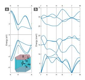
Fig. 2. (a) DFT calculated electronic bandstructure for t-Se showing a direct bandgap of 1.9 eV at the H point and (b) phonon dispersion. Inset shows the brilloiun zone for t-Se.
