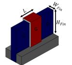
Fig. 2. Structure of the n-FinFET studied in this work.
