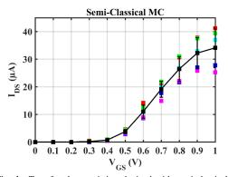
Fig. 4. Transfer characteristics obtained with semi-classical MC simulator for five devices with different random dopant distribution in the source, drain and channel. The average channel doping is  $10^{15}$  cm<sup>-3</sup>. Solid line is the averaged characteristic.  $V_B = V_S = 0$  V and  $V_{DS} = 0.1$  V.
