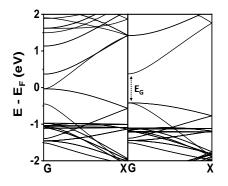
Fig. 2. Band structures of (left)  $In_{0.5}Ga_{0.5}As$  and (right)  $In_{0.5}Ga_{0.5}As$  with DFT-1/2 technique.  $E_G$  is the band gap.
