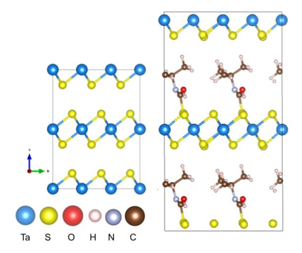
$\begin{array}{lll} Fig. \ 1. & Left: \ pristine \ 2D \ structure \ of \ TaS_2. \\ Right: \ CBOSs-functionalized \ TaS_2 \ structure \end{array}$
