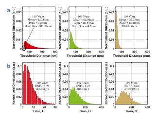
Fig. 5. (a) Threshold distance distributions and (b) avalanche gain distribution for 500 nm *a*-Se bulk drift lengths for electric field strengths of 140, 162 and 196 V/ $\mu$ m, respectively.
