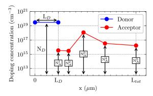
Fig. 1. Sketch of the doping profile structure. The N side is described by its length and level, while the P side is described by a piecewise exponential function defined by  $n_A$  acceptor levels (here  $n_A=5$ ). The x coordinate of the points are not optimized and are chosen to be well distributed. The total number of variables to optimize is  $N_{opt} = n_A+2$ .
