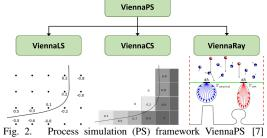
Process simulation (PS) framework ViennaPS [7] including a level set (LS) surface definition, a cell set (CS) volume description, and a ray tracer for physical modeling.
