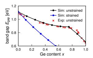
Fig. 2. Comparing the calculated average band gap of unstrained and biaxially strained random SiGe alloys in ralation to Ge content. Red crosses show measurements by Braunstein et al. [2] in good agreement with our simulations.
