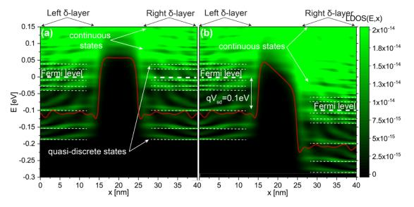
Fig. 3. Local density of state (LDOS) for  $\delta$ -layer tunnel junction device shown in Fig. 1: (a) for an applied of 1 mV; (b) for an applied of 100mV. The semi-quantized states in the conduction band are indicated with dashed lines.
