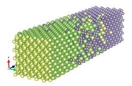
Fig. 2. Ge/GaAs junction with concentration mixing
