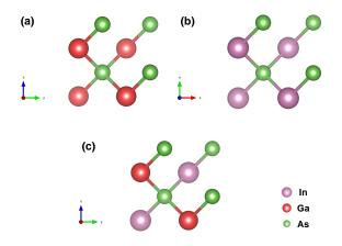
Fig. 1. Atomic structures of conventional unit cells of (a) GaAs, (b) InAs (c)  $In_{0.5}Ga_{0.5}As$ .
