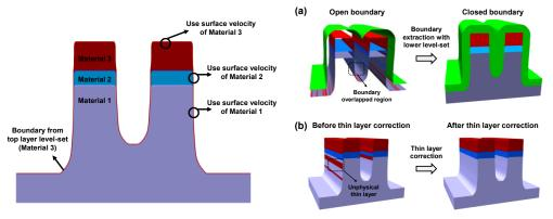
Fig. 1. Schematic of the multi-level-set method. It is shown in which surface velocity is used in the time evolution based on the top layer level-set.
