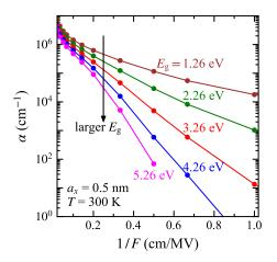
Fig. 2. Impact ionization coefficients  $\alpha$  as a function of inverse electric field for different  $E_{\rm g}$ .  $a_x = 0.5 \,\mathrm{nm}$  and  $T = 300 \,\mathrm{K}$ .
