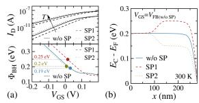
Fig. 6. Simulation results of multi-channel BG CNTFETs with and without different Schottky points. (a) Top: transfer characteristics (300 K and 500 K) at  $V_{\rm DS} = 0.2$  V; bottom: potential barrier height versus  $V_{\rm GS}$  obtained with 1D LBM. (b) Conduction bands at the  $V_{\rm FB}$  of the device without SP. Further details in [4].
