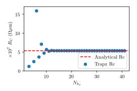
Fig. 4: Convergence of the contact resistance calculated using trapezoidal integration of the transmission coefficient, with varying number of samples in the transverse  $(k_y)$  direction. The analytically calculated value is shown as the dashed red line.
