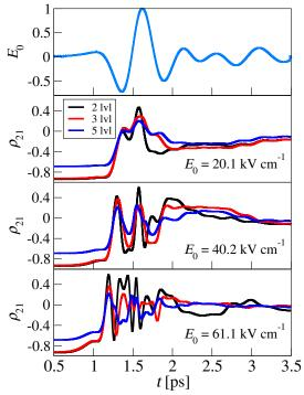
Fig. 4: Top: Experimental input signal generated at resonance of ~ 2 THz presented with normalised amplitude that can be varied experimentally and within the model. Bottom: Population inversion at different input field amplitudes when 2,3 and 5 levels are considered in model in Eqs. (1) and (2). Quantum system parameters are calculated for the structure in Fig. 3, displaying dephasing time  $\tau_{||21} = 0.6$  ps.
