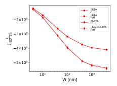
Fig. 3. Comparison between effective RTA and beyond-RTA heat fluxes for AC nanoribbons and the respective Monte Carlo obtained mean fluxes—RTA and bRTA, respectively—for a  $0.2 \,\mathrm{K \ nm^{-1}}$  gradient in the unbound direction. Reproduced from Ref. [9].
