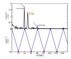
Fig. 2: Experimental probe reflectivity spectrum (top), obtained using a reflection-mode ASOPS geometry, and folded dispersion of the first Brillouin zone (bottom), obtained by solving Eq. (1) for a single period of the Hybrid THz QCL [2].
