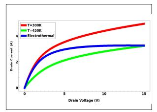
Fig. 5. Output characteristics of the JFET using electrothermal and at fixed temperatures (300K, 450K) at  $V_{\rm gs}$  = 0V.
