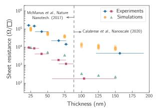
Fig. 4. Extracted sheet resistance for graphene as a function of the channel thickness compared with experimental results obtained in Refs. [1] and [2] before (diamonds) and after (squares) annealing. Two different filling factors FF = 0.35/0.3 for Refs. [1] and [2] and FF = 0.7 are considered in the simulations to reproduce the pre- and after-annealing scenarios. Figure from Ref. [3].
