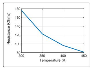
Fig. 6. Sensor resistance as a function of temperature
