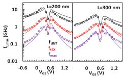
Fig. 4. Intrinsic, extrinsic cut-off and extrinsic maximum oscillation frequencies  $f_{tINT}$ ,  $f_{tEXT}$ ,  $f_{max}$ , respectively for two GFETs with W=24  $\mu$ m and L=200 nm (left subplot), L=300 nm (right subplot) vs. V<sub>GS</sub> at V<sub>DS</sub>=0.5 V. Markers: measurements, lines: model.
