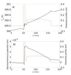
Fig. 3. a) Non-equilibrium electron temperature along the device and b) corresponding electrochemical potential when applying lattice temperature gradient of 1 K and no potential bias (V = 0 V).
