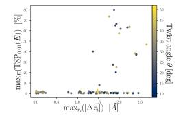
Fig. 5. Spin-polarisation coefficient  $\text{TSP}_{0.01}$  where  $\text{TSP}_{\delta}(\epsilon) = |\frac{T_{\uparrow}(\epsilon) - T_{\downarrow}(\epsilon)}{T_{\uparrow}(\epsilon) + T_{\downarrow}(\epsilon) + \delta}|$ , versus maximal out-of-plane buckling relative to average z of each structure. Maximum taken for -0.5 eV < E < 0.5 eV. 146 points in plot.
