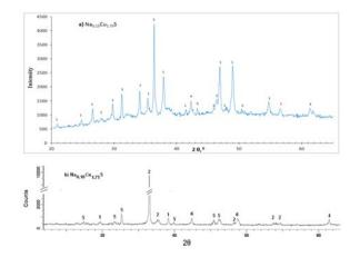
Figure 1. Powder diffraction pattern of the  $Na_{0.15}Cu_{1.75}S$  (a),  $Na_{0.10}Cu_{1.75}S$  (b) samples taken at room temperature. Digits above pikes denotes: 1-triclinic roxbyite, 2–orthorhombic anilite, 3-monoclinic  $Na_2Cu_4S_3$ , 4-cubic  $Cu_2O$ , 5-monoclinic chalcocite  $Cu_2S$ , 6-orthorhombic  $Na_2S$ .
