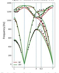
Fig. 3. Phonon dispersions computed from Density Functional Perturbation Theory (DFPT) using Quantum Espresso (red) and from Valence Force Field (VFF) model (green). The DFPT phonon structure is computed using a BLYP functional and optimized norm-conserving Vanderbilt pseudopotential input.
