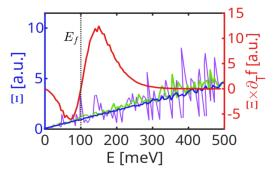
Fig. 5. Transport distribution function using the MC algorithm. The red line (right axis) shows the product of  $\Xi(E)$  and the differential Fermi function with respect to temperature  $\partial_T f$  (shown for the case of 10<sup>4</sup> electrons).
