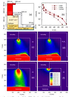
Fig. 4. (a) Sketch of the 2D diode. (b) I-V curve. Color maps of electron concentration for an applied voltage of -30 V in the area delimited in (a) by the dashed rectangle using: (c) air and (d)  $Si_3N_4$  as passivation dielectrics. (e) Electron and (f) hole concentration for V= -40 V and air as dielectric.
