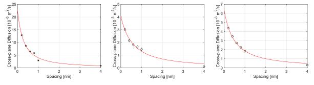
Fig. 3. Effect of additional intertube spacing on cross-plane diffusion constants for three different morphologies of CNT array. Parallel refers to aligned CNTs, "Single Random" refers to randomly oriented unbundled CNTs, and "Bundled Random" refers to randomly oriented bundles of seven CNTs (hexagonally packed) [1].
