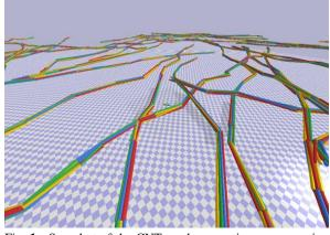
Fig. 1. Snapshot of the CNT mesh generation process using Bullet Physics [1-2]. Each CNT is composed of several segments that are connected together via cone constraints.
