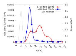
Fig. 4. Probability current at t = 500 fs. The case  $t_1 = 10$  fs (red) clearly shows the presence of significantly different velocities (energies) in the state.
