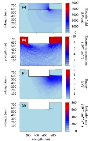
Fig. 3. Maps of (a) electric field modulus, (b) electron concentration, (c) total energy, and (d) II rate obtained with a front-view MC simulation using  $N_D=5\times10^{18}$  cm<sup>-3</sup>,  $\kappa_r=1$  and T=300 K, for a bias of 25 V.
