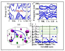
Fig. 6. Matrix element extraction in a complex band material  $Mg_3Sb_2$ . (a-b) Electronic and phononic structure. (c) Three dominant transition types. (d) Matrix elements for each transition type involving all phonon branches.
