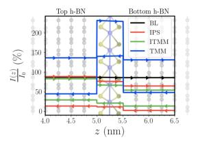
Fig. 2. Net forward and backward propagated energy flux vs. depth in the active region for  $\lambda_0 = 561$  nm. Multiple reflections and interference have strong impact on the overall intensity inside material layers. vdW gaps were not included for the sake of clarity, and  $n_b = n_t = 20$  and  $t_s = 270$  nm were used.
