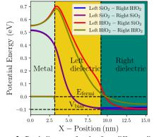
**Figure 2.** Band diagrams for the four different dielectric combinations, obtained by taking the cutlines (along the length of metal and TMD) of the mean of the self-consistent potential along the transverse direction (y). Systems with low- $\kappa$  environment near the metal edge have lower barrier heights and smaller depletion widths.
