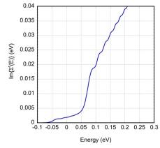
Fig. 1. Imaginary part of the self-energy in Si at 50 kV/cm and 300K.
