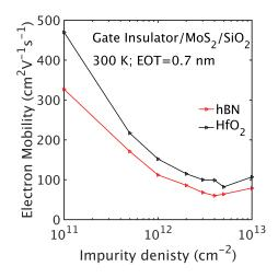
Fig. 2. Impurity-limited mobility vs. impurity density in the hBN/MoS<sub>2</sub>/SiO<sub>2</sub> and HfO<sub>2</sub>/MoS<sub>2</sub>/SiO<sub>2</sub> stacks at 300 K.
