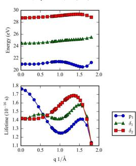
**Fig. 3** Plasmon dispersion (top) and lifetime (bottom) obtained from the position and width of the quasi-Lorentzian peaks  $(p_1, \delta_1, \text{and } \delta_2)$  shown in Fig. 2.
