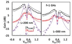
Fig. 5. Intrinsic, extrinsic small-signal current gain and unilateral power gain  $|h_{21INT}|$ ,  $|h_{21EX}|$ , U, respectively for two GFETs with W=24  $\mu$ m and L=200 nm (left subplot), L=300 nm (right subplot) vs. V<sub>GS</sub> for f=1 GHz at V<sub>DS</sub>=0.5 V. Markers: measurements, lines: model.
