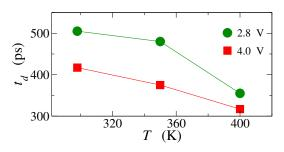
Fig. 4. Simulated delay time  $t_d$  as a function of the lattice temperature T for two plateau voltages (2.8 and 4 V);  $t_d$  is the time interval between the instant at which the applied voltage exceeds the threshold value and the instant at which a steep rise in the device current begins [7], [11], and is a useful parameter for quantifying the switching speed of the electric response.
