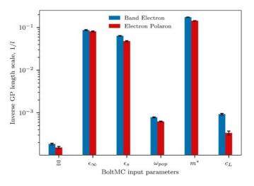
**Figure 1.** Inverse length-scales of the covariance function for each simulation input parameter, plotted such that larger values indicate larger output (mobility) sensitivity to that parameter. Error bars show standard error in the mean in black.  $\Xi$  is the acoustic deformation potential,  $\varepsilon_{\infty}$  ( $\varepsilon_s$ ) the high (low) frequency permittivity,  $\omega_{pop}$  the polar optical phonon frequency,  $m^*$ the effective mass and  $c_L$  the elastic constant.
