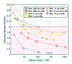
Fig. 4. Plot of ENF from single hole MC simulations for 0.1-15  $\mu$ m *a*-Se bulk drift length as a function of mean gain.
