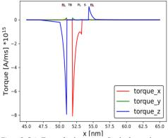
x [nm] Figure 3: Spin Torque for the structure fixed reference layer (RL) - tunnel barrier (TB) - free layer (FL) - spacer (S) fixed reference layer (RL)
