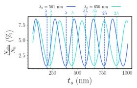
Fig. 6. Normalized  $N_{abs}$  vs.  $t_s$  for two different wavelengths 561 and 650 nm, according to TMM. The period is  $\lambda/2$  in both cases, but resonances do not coincide with multiples of  $\lambda/4$  nor  $\lambda_0/4$  due to additional phase difference introduced by interfaces.
