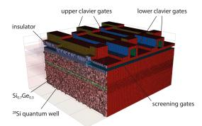
Fig. 2. Boundary conforming Delaunay mesh (generated with TetGen) for computation of the electrostatics problem using the finite volume method implemented in VoronoiFVM.jl [3].
