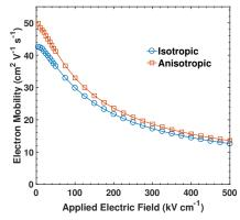
tric field in a bulk Al<sub>4</sub>SiC<sub>4</sub>. The mobility obtained assuming an anisotropic (red squares) and a simpler isotropic (blue circles) bandstructure are plotted.
