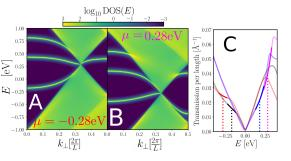
Fig. 4. A-B)  $k_{\perp}$ -resolved DOS for *p*- and *n*-type doping of GB in Fig. 1A. C) The effect of gating on the Transmission through the GB. As the localised state is pushed into the continuum by gating, more electrons can tunnel through the GB. Red:  $\mu = -0.28$ eV, black:  $\mu = -0.17$ eV, blue:  $\mu = 0.18$ eV, magenta:  $\mu = 0.28$ eV.  $\mu$  is measured relative to the Dirac point.
