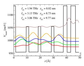
3: Fig. Bandstructure of superlattice  $GaAs/Al_xGa_{1-x}As.$ designed for absorption at 1.94 THz. Conduction band profile and wafefunction moduii squared The are presented. layer structure is 28/80/20/71/20/80/20/71/28/28/36/28, barriers are shown in bold text (x=0.11 and 0.2) and underlined wells are doped by  $2 \text{ cm}^{-1}$ .
