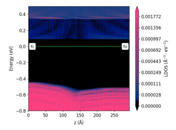
Fig. 3 LDOS of InP interface between Zincblende (on the left) and Wurtzite (on the right).
