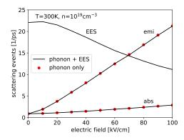
Fig. 1. Number of scattering events in a given time interval versus electric field for phonon emission, phonon absorption, and EES. Two simulations with and without EES are compared.
