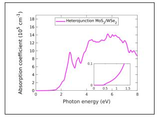
Fig. 2. Absorption coefficient of the MoS<sub>2</sub>/WSe<sub>2</sub> heterojunction, computed with DFT calculation. The inset plot is a zoom in the low energy range.
