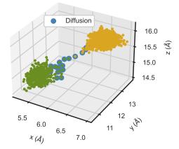
Fig. 1. Example of the performance of our unsupervised algorithm at extracting the diffusive path for one random particle of a DFT-AIMD simulation of  $Li_7La_3Zr_2O_{12}$  at a temperature of 400K.
