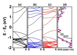
Fig. 5. Band structures of  $In_{0.5}Ga_{0.5}As$  (a) defect-free, (b) w/  $As_{In}$ , (c) w/  $As_{Ga}$  and (d) their density of states (DOS).
