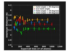
Fig. 2. Average interlayer distance as a function of supercell size. Typically, a supercell containing  $\sim 1000$  atoms is necessary for well-converged simulations.
