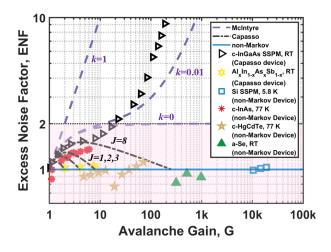
Fig. 1. Excess noise factor in *a*-Se compared with Markov, non-Markov and Capasso type devices.
