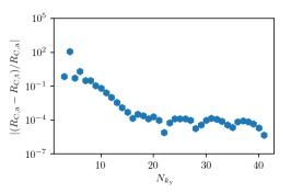
Fig. 5: Convergence of the relative error in the contact resistance between the trapezoidal and analytical integration methods for the transmission coefficient.
