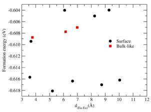
Fig. 3. The formation energy of Eu-doped GaN NW with the variation of Eu distance in NW.
