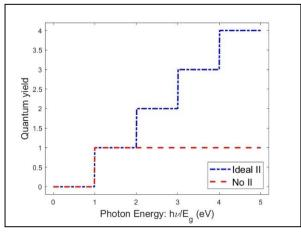
Fig. 1. The quantum yield (QY) is shown as a function of  $hv/E_g$  where hv is the photon energy and  $E_g$  is the gap of the semiconductor. The blue curve shows the QY under ideal impact ionisation (II) and the red curve shows the QY without II.
