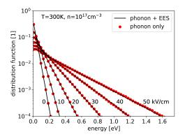
Fig. 3. Distribution functions for uniform electric field at different field strengths. EES has no visible influence.
