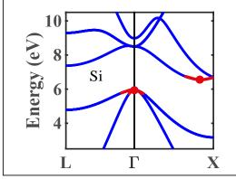
Fig. 1. Electronic structure of Si with relevant transport regions indicated in red [1].
