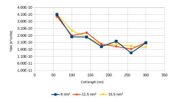
Fig. 4. Thermal boundary resistance dependence on cell length and cross section. A fixed thermal bias of 100K, centered at 300K, has been imposed in every simulation
