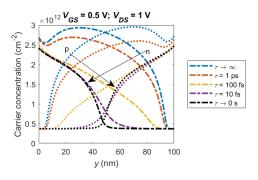
Fig. 4. Electron (dashed-dotted lines) and hole (dotted) concentrations in the channel at Dirac bias for different recombination times.
