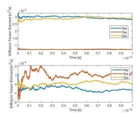
Fig. 2. Mean squared displacements vs. time for each of the components of the diffusion tensor. The diffusion tensor is the long time limit of these plots.
