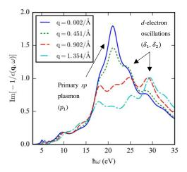
**Fig. 2.** Imaginary part of the inverse dielectric function of GaN calculated using the DFT package Quantum ESPRESSO. The function  $\text{Im}[-1/\varepsilon(\mathbf{q}, \omega)]$  is plotted vs. the energy,  $\hbar\omega$ , for the indicated values of **q**. Plasmon peaks  $(p_1, \delta_1, \text{ and } \delta_2)$  are indicated.
