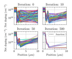
Fig. 2. Illustration of the PSO algorithm where each line represents a particle of the algorithm. The initial population is randomly generated (Iteration 0) and then evolves during the optimization process in order to find a global minimum. For visualization purposes, the N+ length  $L_D$  was kept constant.
