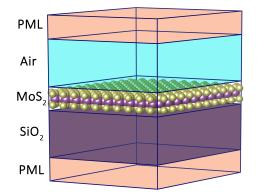
Fig. 1. Schematic of the three-dimensional (3D) simulation geometry of monolayer  $MoS_2$  between air on top and  $SiO_2$  substrate on bottom. The vertical boundaries have periodic boundary conditions.
