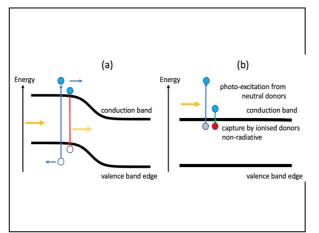
Fig. 2. Band edge profile of (a )solar cell; (b) photo-excited compensated semiconductor
