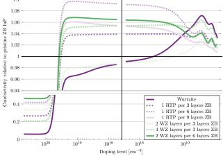
Fig. 6 Conductivity of InP systems along  $[1 \ 1 \ \overline{2}]/[1 \ 0 \ \overline{1} \ 0]$ , relative to pristine ZB InP, at zero bias voltage.
