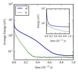
**Fig. 4**. Relaxation of electrons from a kinetic energy of 100 eV shown with the average energy of the generated holes throughout the thermalization process. **Embedded figure:** the first  $10^{-15}$  s of the simulation.
