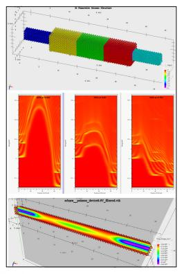
A silicon nanowire FET with 20 orbitals per atom and 8 000 atoms with modespace and electron-phonon scattering: visualization of the NEGF results with Victory Visual Top: NWFET structure with spacers Middle: Density of States resolved in space and energy for different grid voltages Bottom: Free charges in the NWFET
