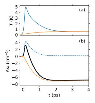
Fig. 1. Transient changes induced in CO/Pd(111) by a 450 nm pump pulse (100-fs duration and absorbed fluence of 40 J/m<sup>2</sup>) that hits the surface at t = 0.1 ps. The initial temperature is 100 K. (a) Electron  $T_e(t)$  (blue) and lattice  $T_l(t)$  (orange) temperatures calculated with TTM. (b) Transient frequency shift of the CO IS mode: black line is  $\Delta \omega(t)$  and dashed blue and orange lines are the contributions of the NC and EMPPC, respectively.
