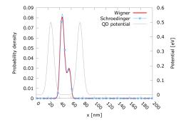
Fig. 1. Probability density of the superposition state at  $t=250~{\rm fs}$ : Comparison between Wigner and Schrödinger. The two peaks of the captured electron state oscillate with  $T\approx500~{\rm fs}.$
