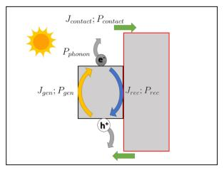
Fig. 4. Carriers fluxes and power flux densities displayed on the band diagram of the device. We consider an isolated system. Thus, carrier exchanges occur only between the small gap heterojunction and the reservoir.
