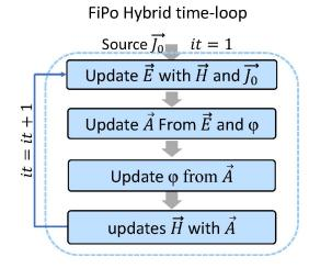
Fig. 1. Flowchart of the  $\phi$ , **E**, **A**, and **H** time-stepping loop for the FiPo Hybrid algorithm. Field and potential updates are consecutive. Arrows show the progression of field or potential values through the update equations.
