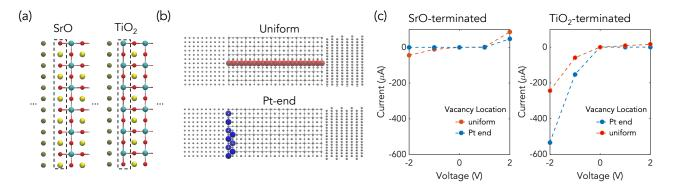
Fig. 2. (a) Atomic structure of a SrO- (left) and a  $TiO_2$ -terminated (right) Pt-SrTiO\_3-Ti stack. (b) Uniform distribution of vacancies (top) and accumulation of vacancies at the Pt electrode (bottom). (c) I-V characteristics of the SrO- (left) and TiO\_2-terminated (right) devices for the two vacancy distributions shown in (b).
