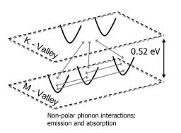
leys for Al<sub>4</sub>SiC<sub>4</sub> showing details of the number of electric field in a bulk Al<sub>4</sub>SiC<sub>4</sub>. The velocity obtained equivalent M- and K- valleys, the separation between assuming an anisotropic (red squares) and a simpler valleys, and the electron-non-polar phonon interac- isotropic (blue circles) bandstructure are shown. tions considered in the transport model.
