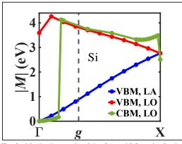
Fig. 3. Matrix elements involving LA and LO modes for the valence and conduction bands in Si [1]. For the CBM and LO mode, clearly the inter-valley nature of the *g*-process is evident (green line is zero close to  $\Gamma$ , and finite close to *g*)
