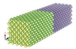
Fig. 1. Ge/GaAs junction with atomically flat interface
