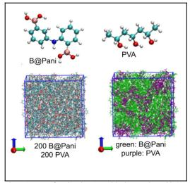
Figure 1: top: B@Pani and PVA models; bottom: box with 200 B@Pani and 200 PVA, ball-and-stick atomic representation and labelling by molecule.
