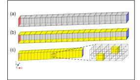
Fig. 2. (a) Nanofilm in cross-plane configuration (CPNF), (b) Nanofilm in in-plane configuration (IPNF), (c) Nanowire (NW) and partial diffusive internal structure for mimicking nanopores. Red/blue faces for hot/cold thermostats  $T_H=302$ K,  $T_C=298$ K, respectively. Yellow faces for diffusive boundaries.
