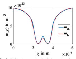
Fig. 3: Self-consistent carrier distribution n dependent on  $\chi$  in a RTD with homogeneous mass distribution  $(m_h)$  and inhomogeneous mass distribution  $(m_{ih})$ .
