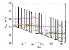
Fig. 4: Conduction band potential of a hybrid QCL design [2] with the addition of the  $30^{\text{th}}$  acoustic mode with modulation M = 5 meV. Two periods are shown at the resonance bias  $K = 3.63 \frac{\text{kV}}{\text{cm}}$  along with the corresponding wavefunction moduli squared.
