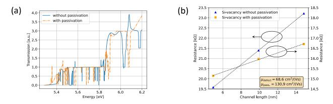
Fig. 3. (a) Transmission function through a  $SiC/SiO_2$  channel with Si-vacancies before (solid line) and after (dashed-dotted line) passivation with nitrogen atoms. (b) Channel resistance as a function of the channel length. Results for the structure with Si vacancies before (triangle) and after passivation (squares) are compared. Lines are guides to the eyes. As expected, a linear resistance increase is obtained. The extracted mobilities with the dR/dL method are reported as inset.
