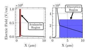
Fig. 3. Electric field at the end of the optimization process that favors depletion. (Right figure is a zoom of the left one.) The device is fully depleted in the absorption region as desired. Yet pushing the electric field within the back of the diode led to a reduction of the thickness of the avalanche region, causing a low breakdown probability (see Fig. 5).
