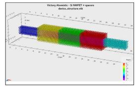
Fig. 1. MOSFET structure of a silicon nanowire oriented [100] with a square cross-section of 3x3 nm<sup>2</sup>.
