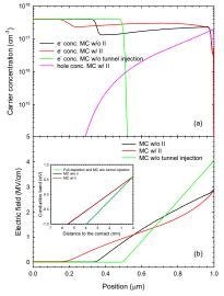
Fig. 3. (a) Profiles of carrier concentration for V=-100 V calculated with and without considering II in MC simulations, as well as without tunnel injection. (b) Corresponding electric field profiles. The inset shows the conduction band at the SC for the same cases (with the metal Fermi level as zero-energy reference) compared with the FD approximation.
