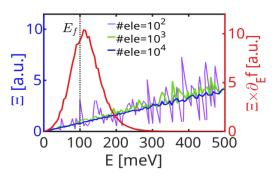
Fig. 4. Transport distribution function,  $\Xi(E)$ , calculated stochastically using the MC algorithm. The red line (right axis) shows the product of  $\Xi(E)$  and the differential Fermi function with respect to energy  $\partial_E f$  (the case of 10<sup>4</sup> electrons).
