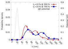
Fig. 2. Evolution along the channel of the electron superposition state ejected at  $t_1 = 10$  fs: Probability density at t = 500 fs and t = 700 fs. The state's peak separation indicates the presence of significantly different velocities (energies) in the state (confirmed in Fig. 4).
