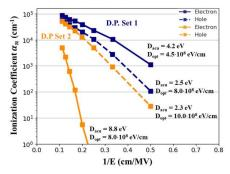
Fig. 4. Impact ionization coefficients from Monte Carlo simulations using two different sets of constant deformation potentials as input. The blue curves use the deformation potential scattering rate (shown in Fig. 2) computed from D.P. Set 1 (inset), and the orange curves use the rate computed from D.P. Set 2 as input. The resulting ionization coefficients are highly influenced by the choice of deformation potential values.
