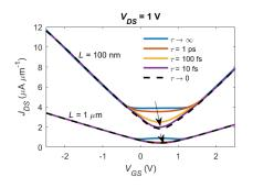
Fig. 2. Transfer curves for different recombination times in GFETs with two channel lengths.
