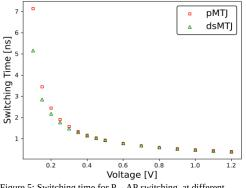
Figure 5: Switching time for  $P \to AP$  switching, at different voltages
