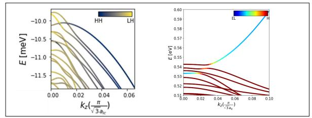
Fig. 3. Left: valence bandstructure of a GaAs/AlGaAs sample with doping density  $1.73 \times 10^{18}$  cm<sup>-3</sup> showing mass inversion. Right: Bandstructure of a InAs/GaSb sample showing band hybridization and the opening of an energy gap induced by the spin-orbit coupling and the self-consistent field. The color respectively indicates the weight of the heavy/light hole or electron/hole character of the states.
