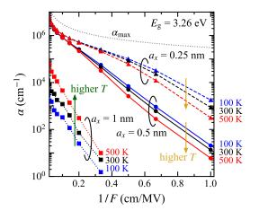
Fig. 1. Inverse electric field dependence of the impact ionization coefficients  $\alpha$  with different BZ widths of  $G_x = 2\pi/a_x$  for  $E_g = 3.26 \text{ eV}$ . Results for T = 100, 300, 500 K are shown by blue, black, and red symbols, respectively.  $\alpha$  for  $G_x = 2\pi/(1 \text{ nm})$  increases with T, while others decrease at higher T. The gray dotted line is the maximum impact ionization coefficient of  $\alpha_{\text{max}} = eF/E_g$ .
