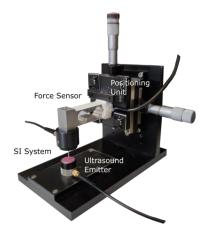
Fig. 2. Measurement Setup with Ultrasound Emitter for SI System Characterization
