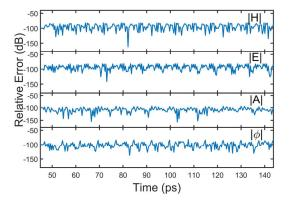
Fig. 2. Relative reflection error for the magnitudes of fields and potentials with CPML implemented for H, E, A, and  $\phi$ . Reference simulation is  $300 \times 300 \times 300$  where the PML is 10 cells thick. FiPo simulation was run on a  $100 \times 100 \times 100$  grid with a PML of 10 cells.
