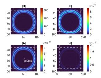
Fig. 3. Visualization of fields and potentials amplitude showing axial x-y cross-section of a 3D simulation domain, sourced by a first derivative of a Gaussian wave packet vector potential (A) at the center and enclosed by an active CPML region, demonstrating the algorithm's vector-potential-sourcing capabilities. FiPo simulation was run on a  $100 \times 100 \times 100$  grid with a PML of 10 cells, z-axis is normal to the plane of the figure.
