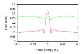
Fig. 3. Fano factor vs. Fermi energy for a graphene sample with W/L = 5 and W = 1000 nm for an ideal sample (red curve) and a disordered sample (green curve)
