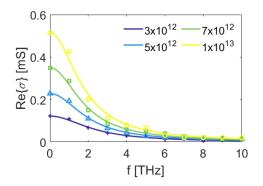
Fig. 2. Real part of  $\sigma(\omega)$  as a function of terahertz frequency for different electron densities in suspended monolayer MoS<sub>2</sub>. The impurity density throughout is  $10^{12}$  cm<sup>-2</sup>. The points are numerically calculated and the solid lines are Drude fits.
