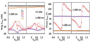
Fig. 1. Magnitude (left plot) and phase (right plot) of deembedded S-parameters (S<sub>DEV</sub>) for two GFETs with gate width W=24  $\mu$ m and length L=200 nm (left subplots), L=300 nm (right subplots) vs. gate voltage V<sub>GS</sub> for operation frequency f=1 GHz at a drain voltage V<sub>DS</sub>=0.5 V. Markers: measurements, lines: model.
