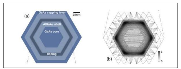
Fig. 1. (a) Cross-section of the GaAs/AlGaAs CSNW illustrating the different materials and the doped region. (b) Example of an optimized FEM grid used to solve the k.p equation of motion with superimposed self-consistent charge density (in grey scale arbitrary units). The grid is limited to the core and first shell, as indicated by the dashed lines.
