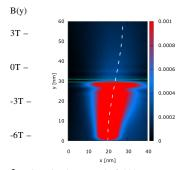
Fig. 3. Case 3: The magnetic field becomes zero at the barrier and switches the sign, giving rise to a snake type of evolution. The density in the upper half of the domain shows again a fine oscillatory structure.
