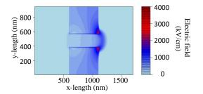
Fig. 2. Map of the electric field modulus obtained with a topview MC simulation using  $N_D=5\times10^{18}$  cm<sup>-3</sup>,  $\kappa_r=1$  and T=300 K, for a bias of 25 V.
