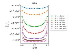
Fig. 1. Fitting to hydrodynamic equation (lines) of RTA-MC calculated heat flux (points) as a function of normalized position for phosphorene AC nanoribbons of different widths under the effect of  $\nabla_{AC}T = 0.2 \,\mathrm{K}\,\mathrm{nm}^{-1}$ . Reproduced from Ref. [9].
