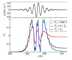
Fig. 1: Top: Secant signal  $E_0^{6\pi} = 63 \text{ MV cm}^{-1}$  that analytically causes three Rabi SIT flops of an ideal two level atom from [1]. Bottom: Population inversion when dephasing time  $(T_2)$  is larger, equal and smaller than signal width  $T_P$ .
