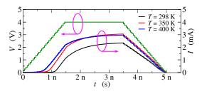
Fig. 2. Currents (right scale) corresponding to a 4-V amplitude and 2-ns plateau duration, at different temperatures. At higher lattice temperatures not only a larger current is obtained, but also the increase in the current occurs earlier: this is due to an increased efficiency of the carrier-heating process at the origin of the OTS effect.
