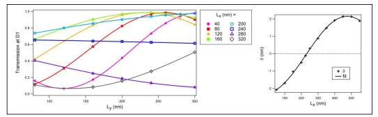
Fig. 3. Behaviour of Aharonov-Bohm oscillations in the interferometer on the right from fig. 1. The transmission probability at D1 (left panel) is reported as a function of the vertical dimension of the *p* region (L<sub>y</sub>) for different values of the horizontal dimension (L<sub>x</sub>). The frequency of the curves changes with L<sub>x</sub>. The right panel shows the distance  $\delta$  between the channels along L<sub>y</sub>, which oscillates as a function of L<sub>x</sub>.
