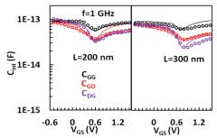
Fig. 3. Intrinsic capacitances C<sub>GG</sub>, C<sub>GD</sub>, C<sub>DG</sub>, respectively for two GFETs with W=24  $\mu$ m and L=200 nm (left subplot), L=300 nm (right subplot) vs. V<sub>GS</sub> for f=1 GHz at V<sub>DS</sub>=0.5 V. Markers: measurements, lines: model.
