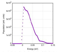
Fig. 3. Distribution function for Si with a field of 50 kV/cm and at 300 K.
