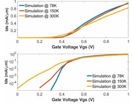
Fig. 3. Simulated transfer characteristics at 78K, 150K and 300K. The applied drain voltage is Vds=0.9V.
