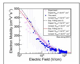
Fig. 2. Electron mobility vs. electric field along [0001] direction. Triangles denote the experimental data from Ref. [5]. The dashed line indicates the model without considering the effect of incomplete ionization.
