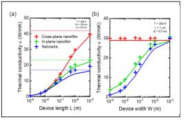
Fig. 4. Thermal conductivity  $\kappa$  as a function of (a) length L with 100 nm width and (b) width W with 1  $\mu$ m length for CP and IP nanofilms and for nanowires at 300 K. Solid and dotted lines represent for semi-analytical models and long-device thermal conductivity, respectively.
