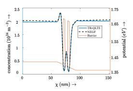
Fig. 4. The electron density from the use of TB-QLTE for one of the both grids is shown as a function of the coordinate  $\chi$  with an applied voltage of 0.05 V. The results are compared to those obtained from the NEGF method. At this point it should be mentioned that the CAP has a considerable influence on the results, so it is important to choose a suitable parameter set for it. Further investigations with regard to the CAP and the boundary conditions will be presented.
