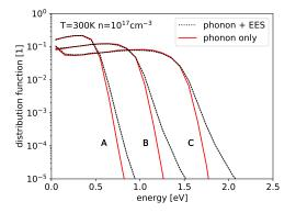
Fig. 6. Distribution functions at positions A, B, C in a  $150 \mathrm{nm}$  channel, calculated with and without EES.
