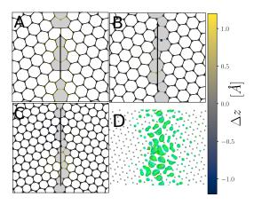
Fig. 1. Examples of bi-crystal grain boundaries with different twist-angle,  $\theta$ . Transport direction is left-right. A)  $\theta = 32.20^{\circ}$ . B)  $\theta = 42.10^{\circ}$ . C)  $\theta = 26.01^{\circ}$ . D) Quasi-particle state (cf. Eq. (1)) of GB in panel C with E = +0.23eV at  $k_{\perp} = 0$ .
