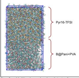
Figure 2: model of the polymer - electrolyte solution interface.
