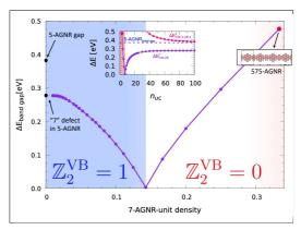
Fig. 1. DFT-SIESTA band gap of 7-(5-AGNR)<sub>nuc</sub> as a function of the density  $(1/n_{uc})$  of 7 widenings for periodic haiku ribbons with supercells containing  $n_{uc}$  5-AGNR unit cells. The band gap closes separating the topological and the trivial phases. The inset highlights the presence of a defect level localized around isolated 7-widenings for very dilute systems. Notice that the labels 575-AGNR and 7-(5-AGNR)<sub>3</sub> denote the same system.
