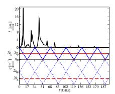
Fig. 3: Experimental probe reflectivity spectrum (top), using the transmission-mode ASOPS geometry, and acoustic dispersion resulting from model in Equation (1) (bottom). Solid blue lines represent the phonon dispersion, folded into the first Brillouin zone. The red dashed line corresponds to  $q = 2k_{\rm L}$ , and the red solid line shows this folded into the first phonon Brillouin zone.
