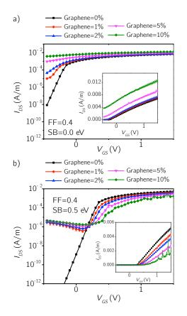
Fig. 5. Transfer characteristics of  $MoS_2$ -graphene composite ink-based printed network device with FF = 0.4 and with a Schottky barrier height of (a) 0.0 eV (b) 0.5 eV. Figure adapted from Ref. [4].
