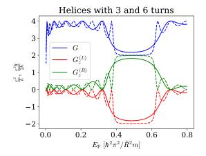
Fig. 3. Charge conductance G and spin left/right spin conductances  $G_z^{(\mathcal{L},R)}$  of a model helical wire with 3 (6) turns are depicted by solid (dashed) lines as a function of the Fermi energy. The helix is attached to non-helical leads.
