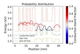
Fig. 1. Carrier probability distribution of lasing states (center), electron injector (left) and hole injector (right) in an interband cascade laser of Ref. [7] simulated by the 8-band  $\mathbf{k}\cdot\mathbf{p}$  solver of the nextnano.NEGF. The color scheme of the wavefunctions signifies the fraction of the conduction-band components in the solutions.
