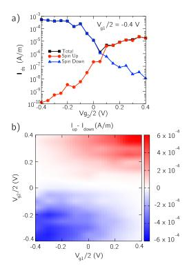
Fig. 2. Total, spin up and spin down currents as a function of  $V_{g2}$  for  $V_{g1}/2 = -0.4$  V. b) Color map of the difference between spin up current ( $I_{up}$ ) and spin down current ( $I_{down}$ ) as a function of  $V_{g1}$  and  $V_{g2}$ .
