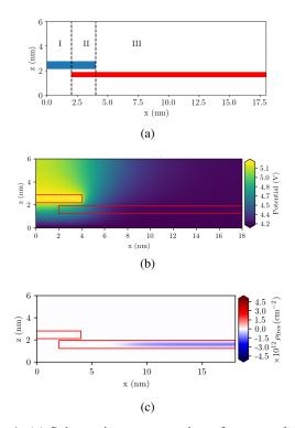
Fig. 1: (a) Schematic representation of our metal-2D semiconductor contact. Self-consistently calculated Hartree potential (b) and free charge density (c). The calculated Schottky barrier is 0.57 eV. We add a sheet doping of  $\rho_{\rm sheet} = 5 \times 10^{12} \ {\rm cm}^{-2}$ .
