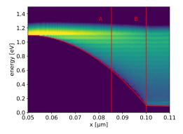
Fig. 4. Potential profile in a 50nm channel. The distribution function shown is calculated assuming phonon scattering only.
