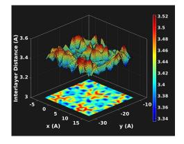
Fig. 4. Average interlayer spacing of the corrugated hBN/hBP heterobilayer twisted at  $\theta = 10$  degrees. The interlayer spacing varies nonlinearly with twist angle, preventing a smooth correlation between  $e_{33}$  and twist angle.
