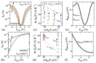
Fig. 3. Extraction of  $\Phi_{\rm SB,eff}$  height of (a), (c), (e) a multitube CNTFET and (b), (d), (f) a multiwire NWFET. Further details on experimental data, plots and related discussions are provided in [4].
