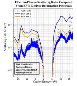
Fig. 2. Electron-Phonon scattering rates computed from EPW-derived deformation potentials, using GW energies and wavefunctions as input (blue). The phonon band structure is computed using DFPT in Quantum Espresso. Both sets of points calculated using a BLYP functional and optimized norm-conserving Vanderbilt pseudopotential input.
