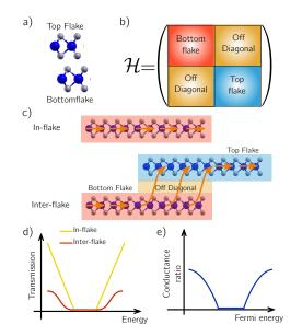
Fig. 3. (a) Bilayer structure used for ab-initio calculations. (b) Schematic wannier Hamiltonian, with indicated the subhamiltoanians for the bottom layer, top layer and the coupling between them (off-diagonal). (c) In-flake and inter-flake structures. (d) Pictorial depiction for the in-flake and interflake transmission coefficients. (e) Schematic depiction of the conductance ratio as a function of the Fermi energy
