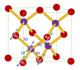
Fig. 1. Motion of the atoms on one basis set may be the LO mode, simultaneously the other atoms in the tetragonal bonding are undergoing TO motion.
