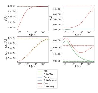
Fig. 2. Electrical conductivity, Seebeck coefficient, total thermal conductivity at zero electric current, and figure of merit as function of NW radius at 300 K and an acceptor concentration (B) of  $1.0 \times 10^{18}$  cm<sup>-3</sup> for several approaches to collision operator; namely, relaxation time approximation or RTA(green), uncoupled beyond the RTA (blue), and dragged (red). Bulk values (dashed) are given as reference.
