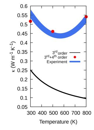
Fig. 1.  $Cs_2NaYbCl_6$  thermal conductivity  $\kappa$  as a function of the temperature. The black line shows the theoretical prediction of  $\kappa(T)$  based solely on cubic anharmonicity. The conspicuous underestimation of the anomalous experimental trend (blue band) is eventually resolved by the inclusion of fourth-order anharmonicity (red points)
