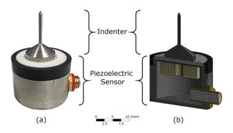
Fig. 1. Sensor-Indenter System – (a) Real Device and (b) Simulation Model (Cut Open)
