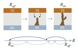
Fig. 1. Schematics of the transition from high- to lowresistance state in an ECM cell. Here, the top (TE) and bottom (BE) electrodes are separated by an insulating layer. Bottom: two different realizations of the resistance switching process.
