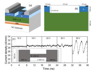
Fig. 1. (a) 3D structure of the simulated device. (b) Longitudinal cut at the etched sides of the channel with an isolation depth of h=174 nm. (c) Time-sequence of the current density for  $N_D$ =5×10<sup>18</sup> cm<sup>-3</sup>,  $\kappa_r$ =1 and *T*=300 K for the single channel device shown in the inset.
