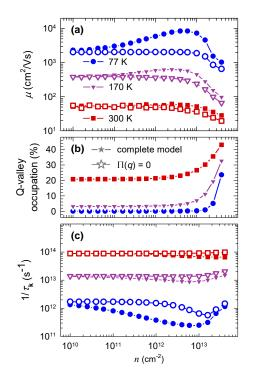
Fig. 1. (a) Low-field electron mobility, (b) upper (Q) valley occupation, and (c) inverse of momentum relaxation time due to scattering mechanisms at three different temperatures in monolayer MoS<sub>2</sub> supported on a SiO<sub>2</sub> substrate. Solid symbols relate to simulations accounting for all the phenomena of the EMC model, and open symbols to results where the screenings due to free carrier is omitted.
