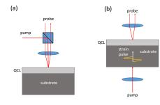
Fig. 1: Schematic illustrations of ASOPS experimental configurations, showing (a) reflection mode, and (b) transmission mode geometries.
