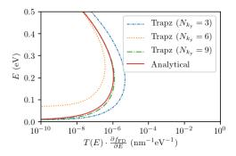
Fig. 3: The transmission coefficient, multiplied by the derivative of the Fermi-Dirac distribution, calculated using trapezoidal and analytical integration of  $T(E) = \int dk_y T(E, k_y)$  for  $N_{k_y} = 3$ ,  $N_{k_y} = 6$ and  $N_{k_y} = 9$ .
