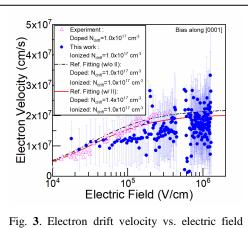
along [0001] direction. Triangles denote the experimental data from Ref. [5]. The dashed line indicates the model without considering the effect of incomplete ionization.
