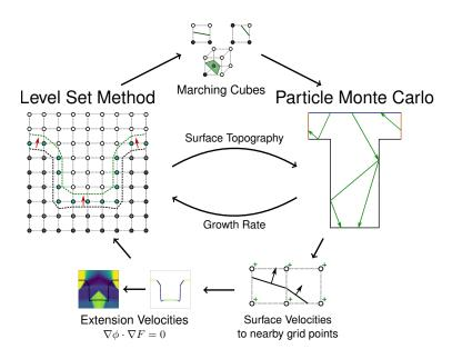
Fig. 2. Geomectric surface growth model: Surface is maintained in the Level Set representation, and is advanced according to the local growth rate sampled from particle Monte Carlo simulations.
