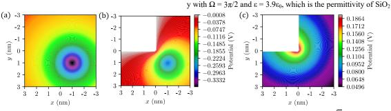
Figure 2: Graphs taken at z = 0 of (a) V<sub>c</sub>, the potential caused by a single electron located at  $(r_0, \theta_0, z_0) = (\sqrt{2}, 3\pi/4, 1)$ , b) V, the potential an electron experiences in the presence of a metal wedge with  $\Omega = 3\pi/2$ , and c) V<sub>I</sub>, the attractive potential exerted by the metal wedge due to the presence of the electron. Note that V<sub>I</sub> = V - V<sub>c</sub>.
