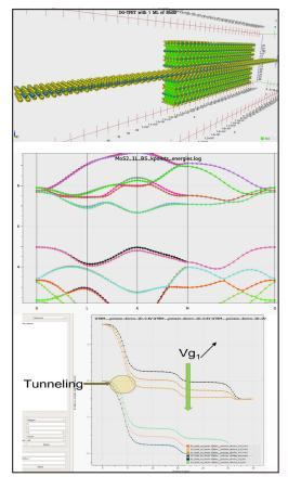
Dual-gate TFET with one monolayer of MoS2 – Top: device structure with insulator (green), Mo (blue) and S (yellow) atoms Middle: Band Structure of the Wannier Hamiltonian Bottom: TFET 1D band profile function of the gate voltage applied
