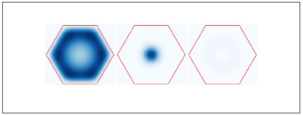
Fig. 2. Electron (left), light-hole (center) and heavy-hole (right) density for the ground of a heavily doped GaAs/AlGaAs sample, with doping density 1.9x10<sup>18</sup> cm<sup>-3</sup>.
