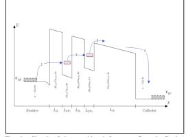
Fig. 1. Sketch of the considered Quantum Cascade Cooler heterostructure under potential bias. The red dashed rectangles represent the QW states, while  $E_{FE}$  and  $E_{FC}$  are the Fermi levels of the emitter and collector respectively. For all the considered devices, doping in the emitter and the collector is  $10^{18}$  cm<sup>-3</sup>.  $L_{BI} = L_{B2} = 6$  nm,  $L_{QWI} = L_{QW2} = 5$  nm,  $L_{B3} = 30$ nm. Blue arrows highlight intended pathway for the electron flow.
