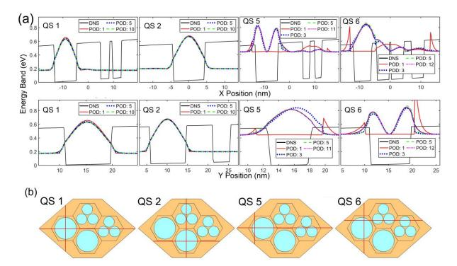
Fig. 3. (a) Profile plots in x (top row) and y (bottom row) for the  $|\psi|^2$  of QSs 1,2,5 and 6 along the horizonal and vertical plotting paths (red lines) shown in (b). The paths were selected to show the maximum probability density in the state.
