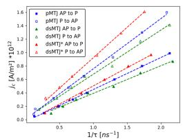
Figure 2: Switching current j\_c for  $AP \rightarrow P$  and  $P \rightarrow AP$  switching respectively. The configuration of the magnetization of the fixed layers was antiparallel (dsMTJ) and parallel (dsMTJ\*)
