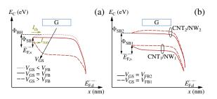
Fig. 2. Conduction band diagrams of a 1D-FET with (a) single-1Dchannel and (b) multi-1D-channels at different  $V_{\rm GS}$  [4].
