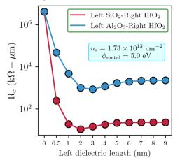
Figure 4. Contact resistance as a function of left dielectric length for metal-WS<sub>2</sub> system. For both cases, we observe an optimal left dielectric length of about 2 nm that gives the lowest  $R_c$ .
