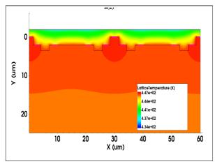
Fig. 3. Temperature profile for  $V_{gs} = 0V$ ,  $V_{ds} = 15V$ ,
