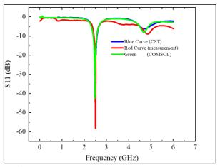
Fig. 2. Measured and simulated  $S_{11}$  vs. frequency curves of the 2.5 GHz rectangular loop antenna defined in figure 1.
