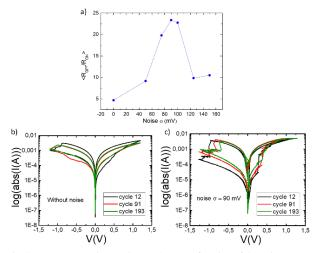
Fig. 2: a) Mean memristor ratio  $R_{OFF}/R_{ON}$  as a function of the noise ( $\sigma$ ). The typical stochastic resonance curve is observed. Memristor I-V curves at cycles 12, 91 and 193 b) without and c) with 90 mV noise  $\sigma$ .
