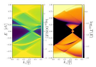
Fig. 3. Out-of-equilibrium  $k_{\perp}$ -resolved density-of-states(left) and transmission function (right) of the GB in Fig. 1C. Chemical potentials set to  $\mu_L = -\mu_R = 0.1$ eV. Presence of Fanotype resonances in the transmission can be seen as black arcs.
