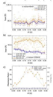
Fig. 5: Current during the 20 cycles for each  $\Delta t$  shift (post-synaptic pulse delay) and mean current evaluated after a set pulse (orange) and after a reset pulse (blue) a) for the case w/o noise and b) adding a  $\sigma = 150 mV$  Gaussian noise. c) Mean resistance ratio versus the post-synaptic pulse delay without noise (blue) and with noise (orange).
