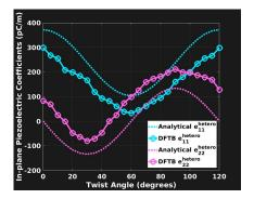
Fig. 3. In-plane piezoelectric coefficients  $e_{11}$  (blue) and  $e_{22}$  (red) vs. twist angle. The solid lines and the dotted lines are the DFTB results and the analytical formulas derived from isolated monolayers respectively.
