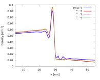
Fig. 5. Density distribution along y-direction, obtained after xintegration of n(x, y): Cases 1&3 and 2&4 clearly group together, suggesting that the oscillations are suppressed in the presence of a magnetic field in the region of the barrier, further indicating that the EM fields interact locally.
