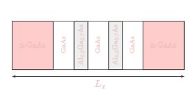
Fig. 2. Structure of a AlGaAs/GaAs resonant tunneling diode with a width of  $L_x$ =152 nm, barriers of 3.38 nm width and a quantum well of 4.5 nm width. The contacts are n-doped with a concentration of  $N_D$ =2 \* 10<sup>18</sup> cm<sup>-3</sup>. A spatially constant effective mass distribution with the effective mass of GaAs is assumed.
