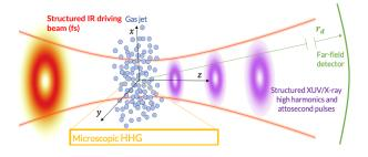
Fig. 1. Scheme of HHG from the macroscopic level. An ultrafast and ultraintense structured IR driving beam is focused in a gas jet. As a result of the highly nonlinear interaction, structured x-ray high-order harmonics, emitted in the attosecond timescale are emitted. The overall emission results from the coherent addition of the dipole acceleration emitted from each atom in the gas target.
