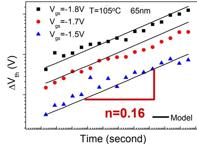
$$\Delta V_{th} = A \left[ (1 + \delta) t_{ox} + \sqrt{Ct} \right]^{2n}$$
