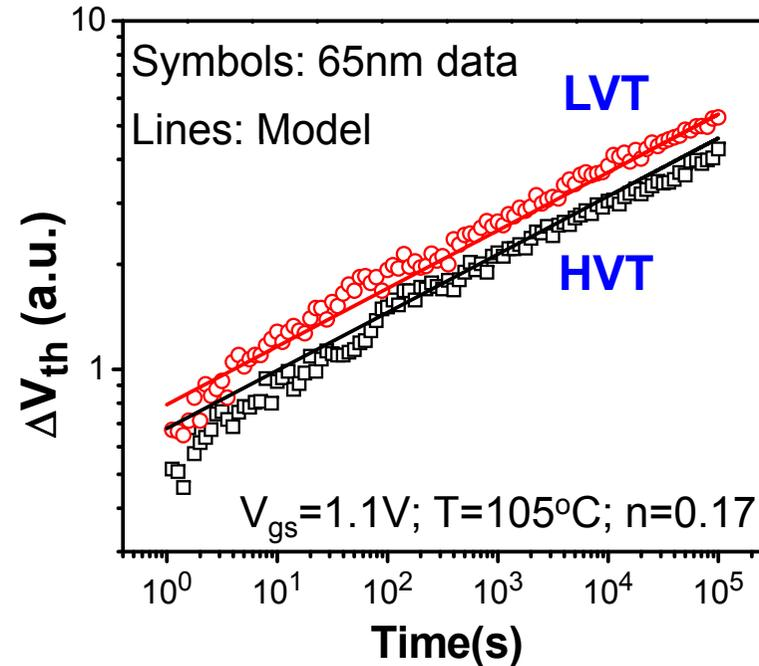
$$\Delta V_{th} \propto Q_i \exp(E_{ox}/E_0)$$
